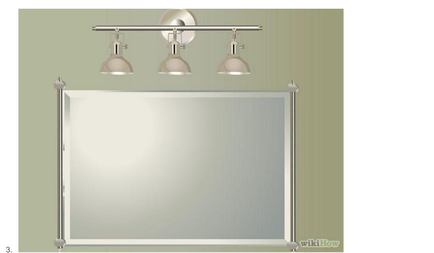
Mount one fixture over the mirror to light a bathroom, but realize it can cause shadows on the face. If using recessed lighting, avoid creating shadows by not mounting them directly over the mirror.
